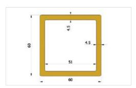
Posts Dimensions: 60 x 60 mm Profile thickness: 4.5 mm Standard length: 6000 mm Colour: yellow or grey Weight: 1.24 kg/m
