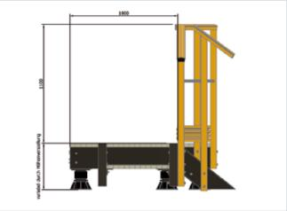
GRP landing composed of GRP profiles as substructure, height-adjustable plastic bases for height compensation as well as a GRP handrail system. These platforms are tailored to the construction requirements of our customers.
