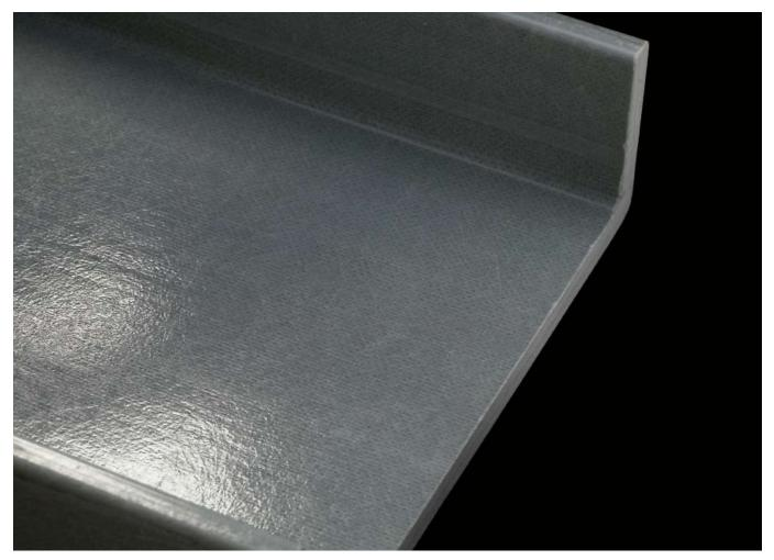
Profiles are produced by means of a pultrusion method. This method is distinguished by a continuous production procedure. The materials used are pulled into the pultrusion machine and shaped into the desired form. The materials are immersed in resin and are then passed through a tool until the final profile shape is achieved. Standard profiles are 6000 mm long.
