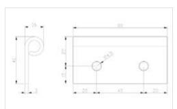
Hinges can be supplied in galvanised steel, stainless steel Wst. 1.4301 and stainless steel Wst. 1.4571.
