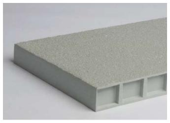
Sandwich panel – model code: GRP–Sandwich A GRP grating which is solid on both sides. A GRP panel is laminated on both the top and the bottom. The surface can be sanded to prevent slipping. Such flooring is especially good in area's if you need close tolerances for flatness.
